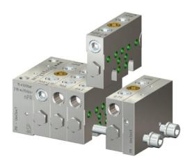
nPr uses an innovative rail & lock concept to allow the element to be replaced or reorganized without the need to completely dismantle the assembly. This is an industry first for segmented progressive dividers allowing quick easy modification or replacement of an assembly element without the cost of a separate base porting module.
